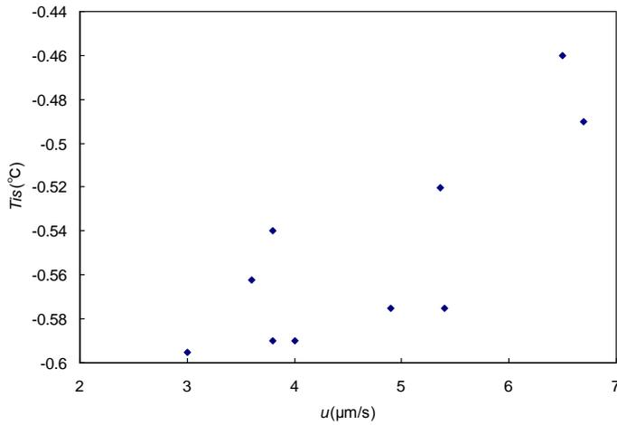
Fig.3 Interface temperature as a function of interface velocity in the case of mixed solution
