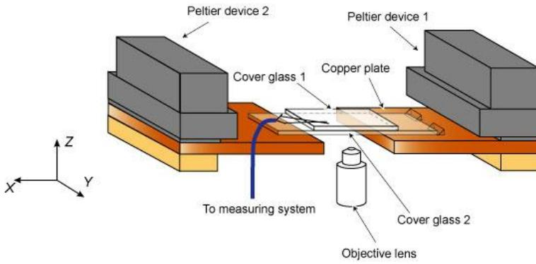
Fig. 1 Details of cooling section
